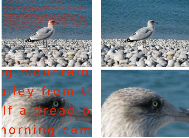
Figure 1: Using dictionary learning to remove overlaid text from images. The authors learned a dictionary A from many natural images, and then removed the text from an image y by (roughly) first representing y as \sum x_k a^k and then zeroing out all the x_i 's that are below some threshold. Photos taken from: J. Mairal, F. Bach, J. Ponce, and G. Sapiro. Online Dictionary Learning for Sparse Coding . In ICML 2009 (See also Mairal, Julien, Michael Elad, and Guillermo Sapiro. "Sparse representation for color image restoration." , IEEE Transactions on Image Processing 17.1 (2008): 53-69 for a clearer description of the method as well as some nice images of how the dictionary looks like that should be added to the scribe notes... )
