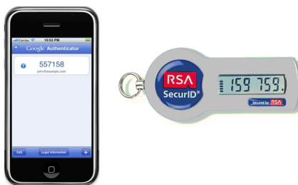
Figure 2: The Google Authenticator app is one popular example of a one-time password scheme using pseudorandom functions. Another example is RSA's SecurID token.
